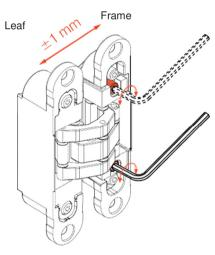
4. Depth adjustment (pressure on the gasket).
